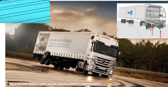
Fig. 3: ESP roll-over control in reality and the respective SIMPACK model simulation
